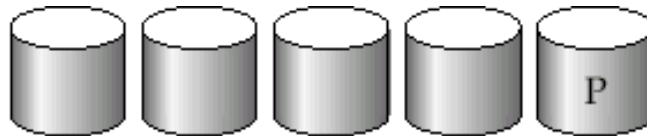
(e) RAID 4: block-interleaved parity
